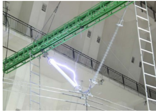
Critical Impulse Flashover Test of 400kV suspension string
