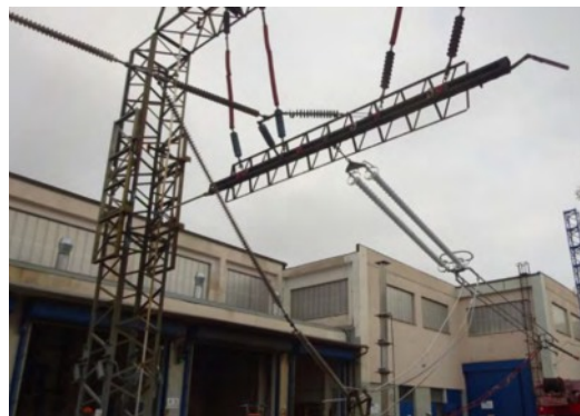
Power Arc Test of 345kV suspension insulator string
