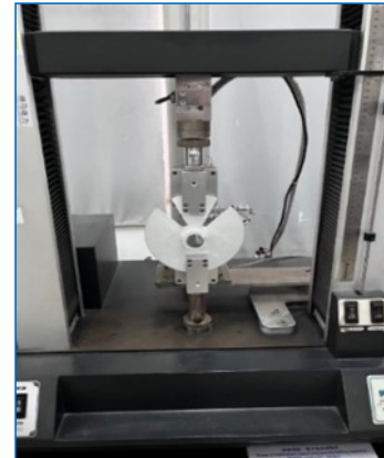
Bonding Pull-off Test
