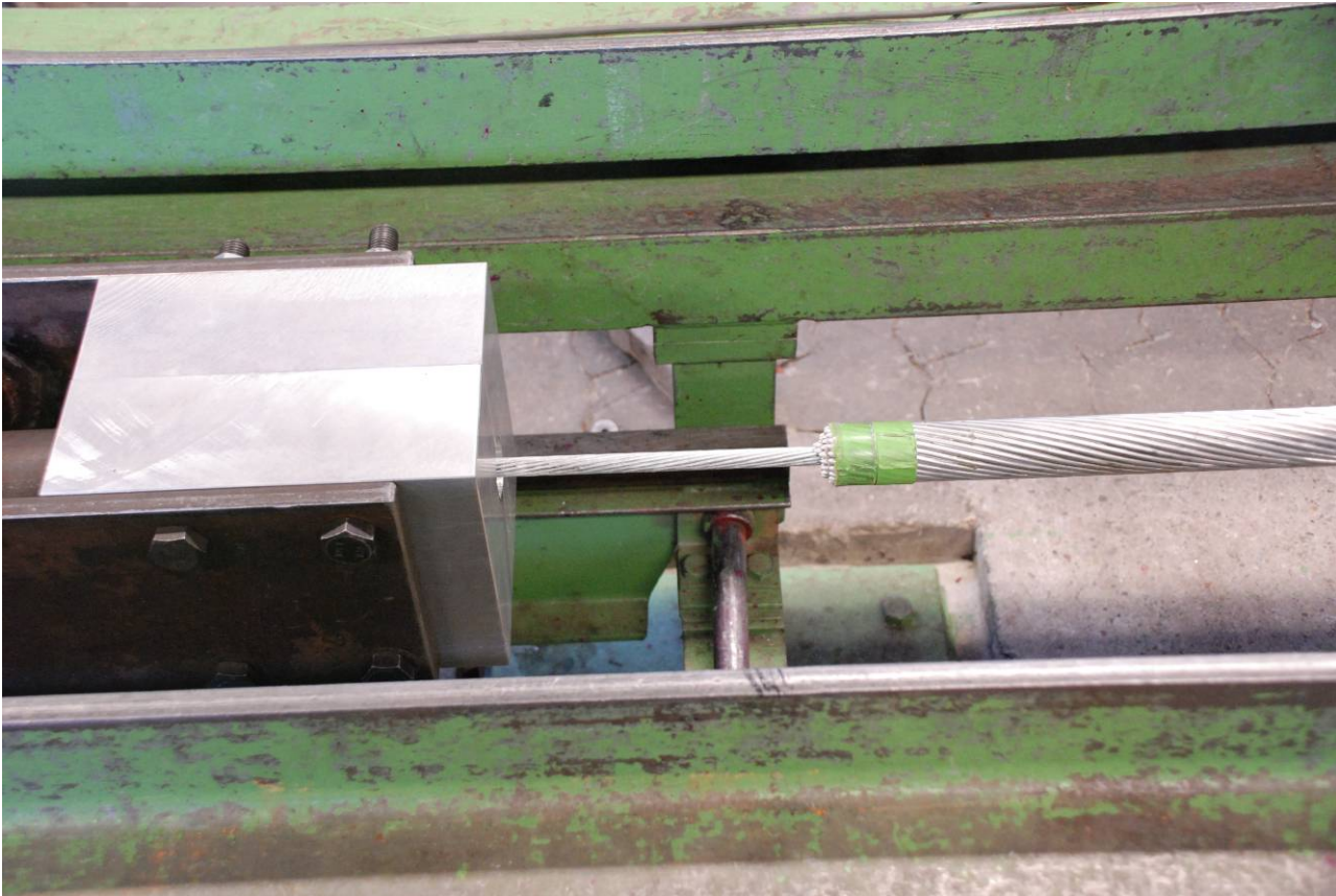
Figure 9 : Breakage of the aluminum at the border of the clamp during the tensile test
