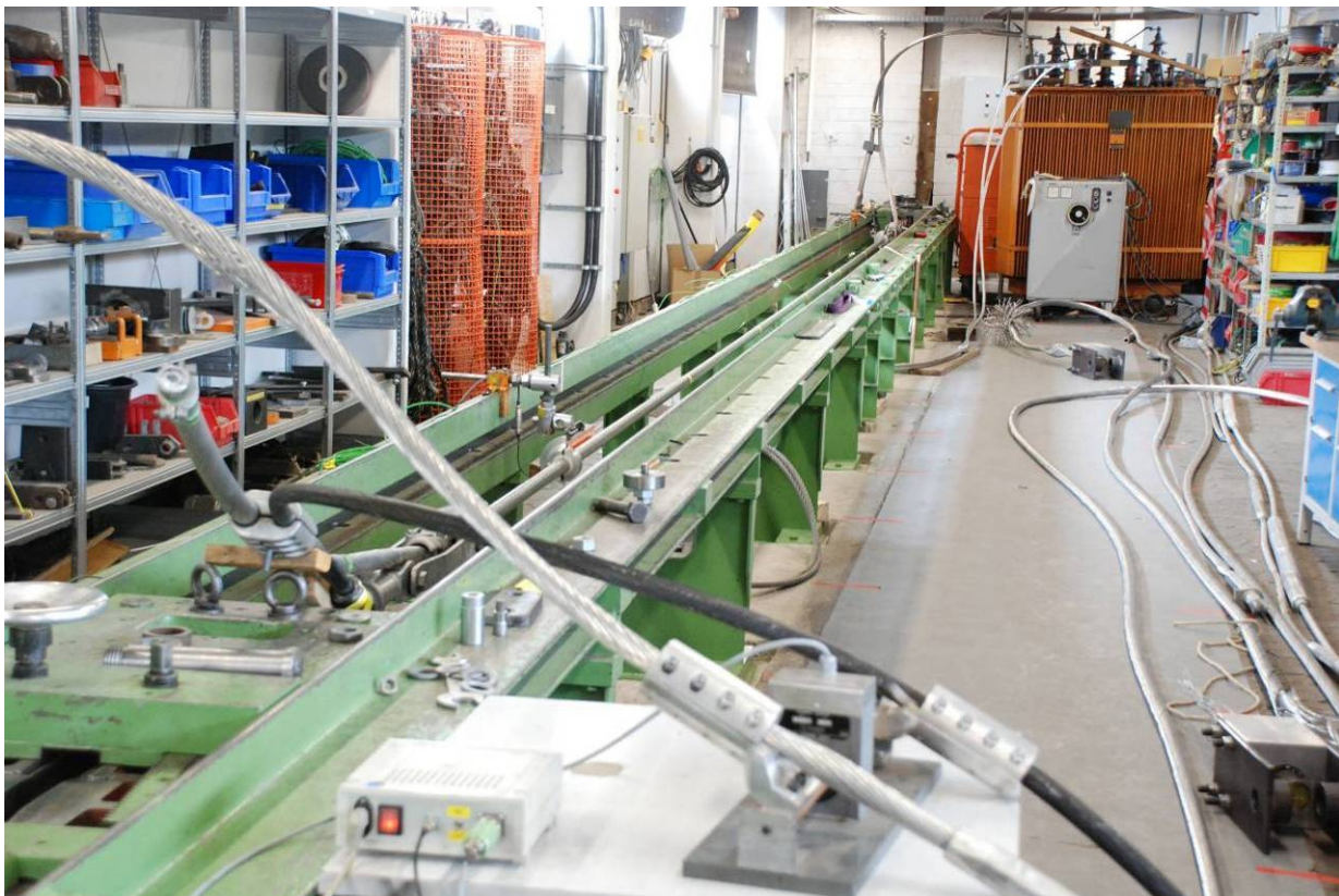
Figure 8 : ACSR Falcon in the tensile machine for the CTE Test
