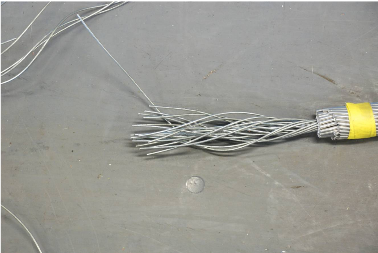
Figure 11 : Breakage after the tensile test on the core
